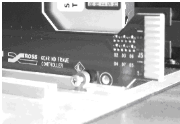
Figure 2.1 MFC-8300 Controller Card and Unscrewed Retaining Screw (MFC-8310 shown)
